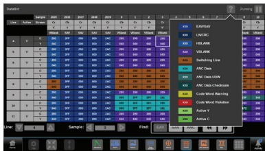
Selecting the question mark within the Datalist display shows the color code legend used to identify certain types of data. For instance the switching line is indicated in brown.
