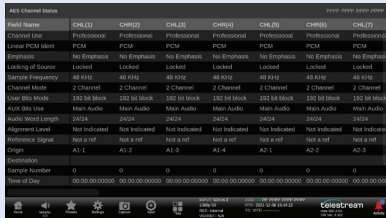
When the Channel Use mode of Professional is used the instrument automatically decodes the syntax as shown above
