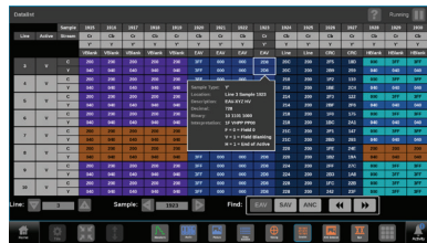
The user can search through the data by line and sample location or use the Find function to search for EAV, SAV or ANC within the signal. Simple pressing the sample will provide a tooltip interpretation of the data.
